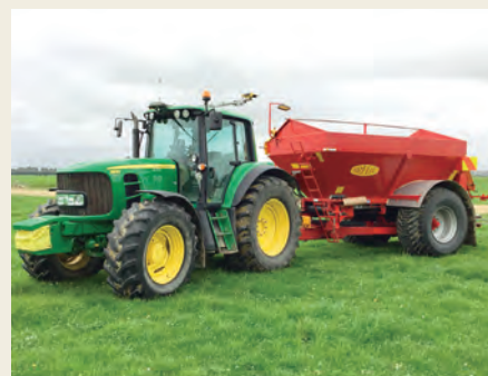
Fertilizer distributor mounted with laser-type sensors and auto-steering system
