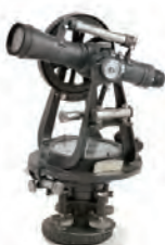
TOHKOH Transit 3-and-half inch, the first surveying instrument manufactured at the main factory at Itabashi
