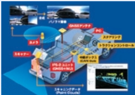
Illustration of IP-S2 system
